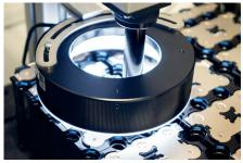
The integrated metrology ensures maximum precision in handling powder press parts.
